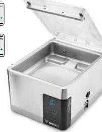
PUMP CAPACITY 21 m³/h MACHINE CYCLE 15-35 sec CHAMBER DIMENSIONS 370 x 420 x 180 mm MACHINE DIMENSIONS 544 x 499 x 461 mm SEAL BAR 420 mm WEIGHT 64 kg VOLTAGE 230V-1-50Hz POWER 0.75-1.0 kW
