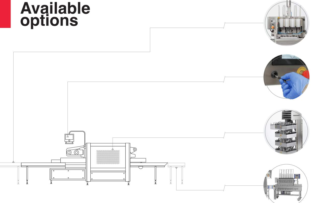
**Use a tray denester** in front of infeed-conveyor for automatic denesting of trays.
