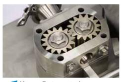
Heavy Duty metering pump Hitec has achieved to make heavy duty metering pumps by stronger drive shaft, stronger idler shaft and more durable bearings. Our design offers excellent long term weight control with less necessary overhauls.
