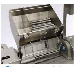
Flapper style casing feed mechanizm The HITEC M-3X features Hitec's unparallel hopper design that eliminates the need for a casing clamp. The design is quick and easy operating and reliable feeding of casings.
